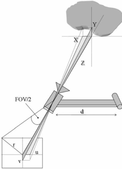
**Figure 2:** A more practical approach to the estimation of the unknown coordinates of a detected point
