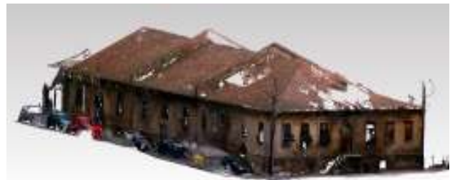
Figure 3. Triangular Mesh produced automatically from the coloured point cloud using Geomagic Studio 9
